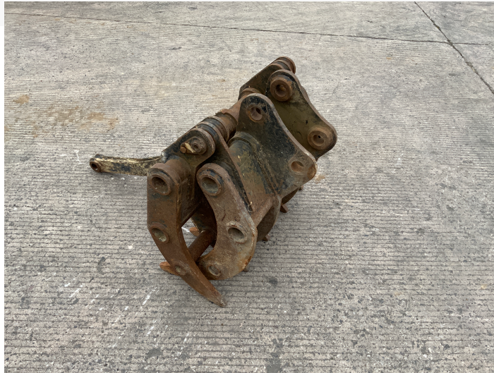
9 FINGER GRAB TO SUITE 8 TONNE EXCAVATOR
