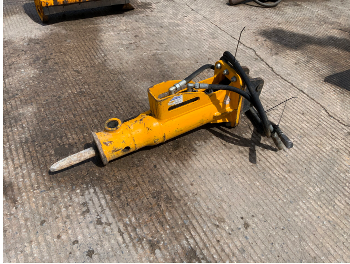
ARROW HEAD BREAKER
