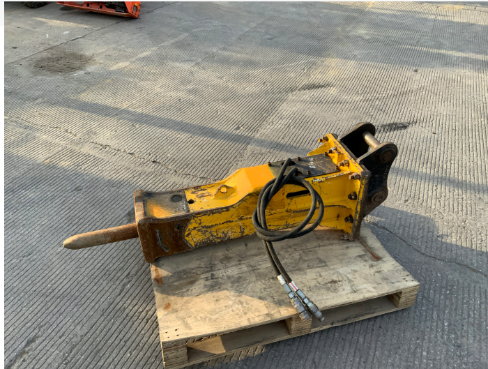
BREAKER TO SUIT 8 TONNE EXCAVATOR
