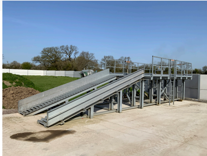
GALVANIZED WASH RAMP
