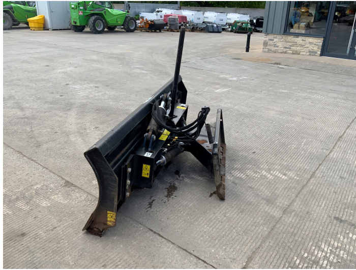
JCB HDB96 DOZER BLADE 8FT 6 WAY HYDRAULIC BLADE (ST26725)
